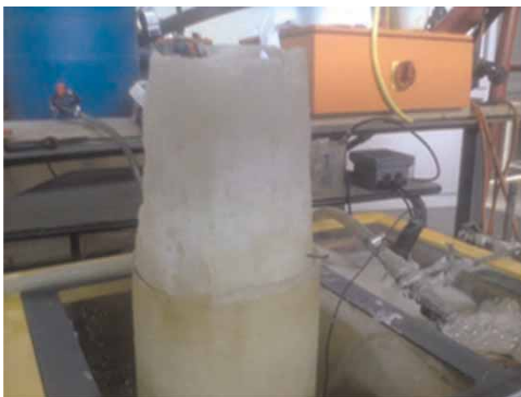
Figure 11 | Ice behaviour in the filter.
