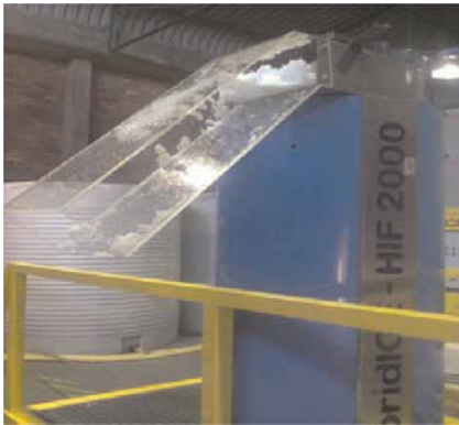
Figure 2 | HybridICE filter in operation (Adeniyi et al. 2013b).
