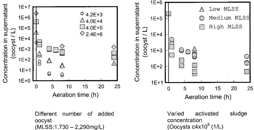
**Figure 1** Relationship between aeration time and oocyst concentration in supernatant**River water**
