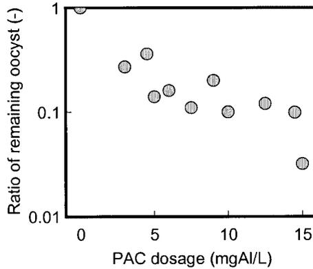
**Figure 3** Effect of PAC dosage on oocyst removal
