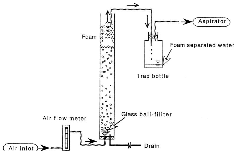
**Figure 1** Schematic diagram of batch foam separating system (not to scale)
