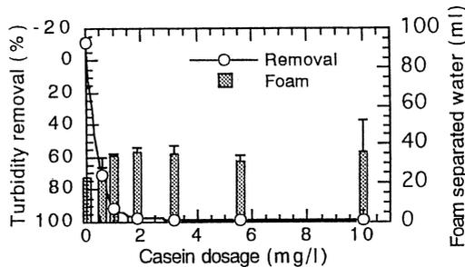
**Figure 3** Turbidity removal and the amount of foam separated water as a function of casein dosage in coagulation and foam separation (FeCl<sub>3</sub>, 20 mg-Fe/L; pH, 5.2(5.8))
