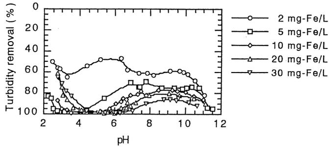
**Figure 2** Turbidity removal by coagulation sedimentation method with FeCl<sub>3</sub> as a function of pH
