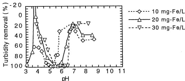
**Figure 4** Turbidity removal as a function of pH in coagulation and foam separation (FeCl<sub>3</sub>, 20 mg-Fe/L; casein, 3 mg/L)
