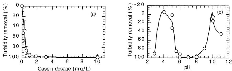
**Figure 5** Turbidity removal by coagulation and foam separation using PAC and casein (a) as a function of casein dosage: (PAC, 20 mg-Al/L; pH, near 7), (b) as a function of pH (PAC, 20 mg-Al/L; casein, 3 mg/L)
