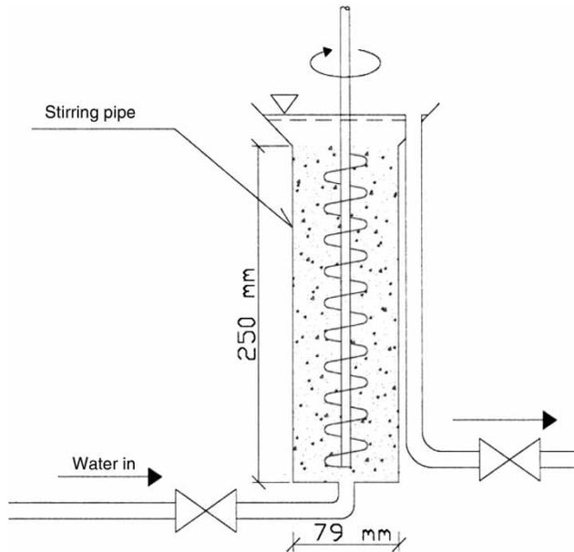
**Figure 2** | Best version of limestone grinder used in pilot tests. Mixing auger diameter 32 mm and speed 180 rpm.
