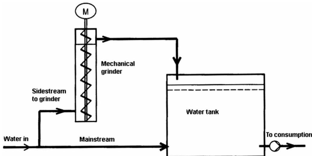
Figure 1 | Schematic diagram of the process involved in including a mechanical grinder in limestone alkalisation of groundwater before consumption. M = motor for auger.
