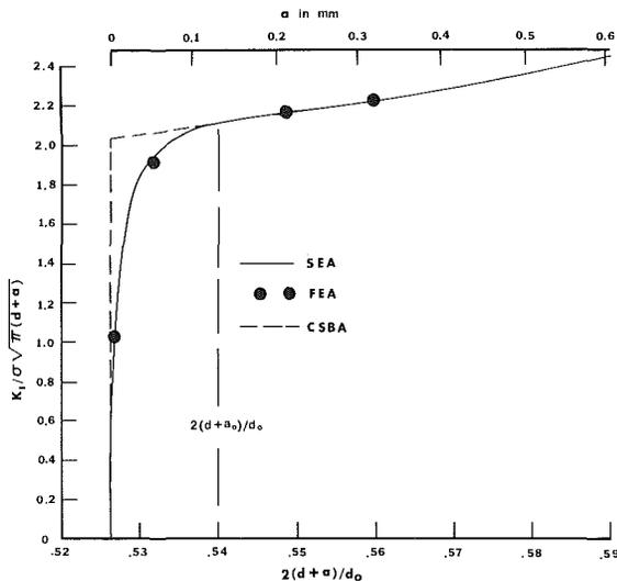
Fig. 4 Stress intensity factor for a circumferential crack emanating from a notch in a round tensile bar
