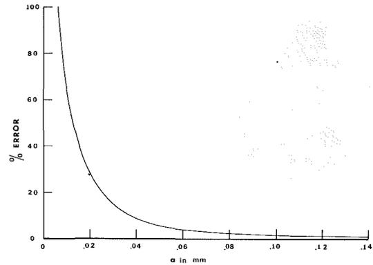
Fig. 5 Stress intensity factor error based on using the cracked-smooth bar assumption
