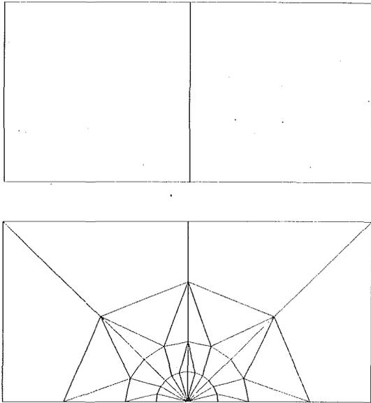
Fig. 3 Lower sketch: Crack tip mesh inserted into base mesh at the crack tip; Upper sketch: Eight noded quadrilaterals inserted at alternate crack tip locations.
