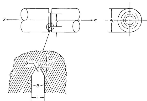
Fig. 1 Cracked-notched round tensile bar
