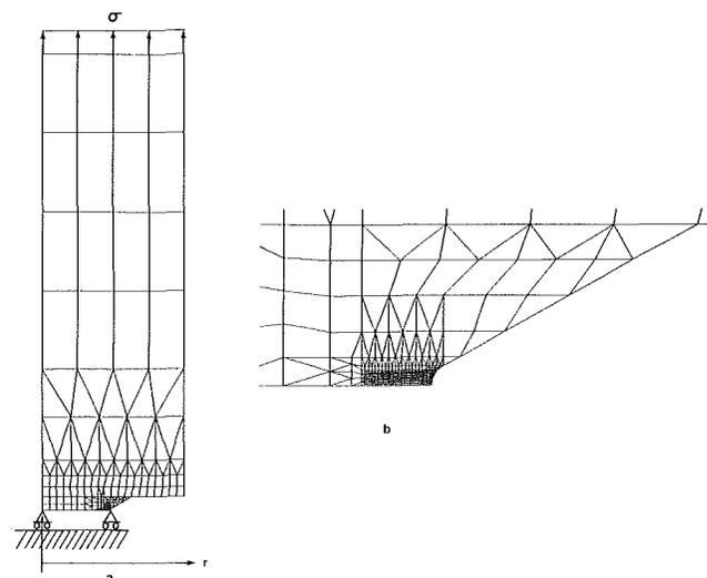
Fig. 2(a) Axisymmetric finite element model; (b) enlargement of notch area
