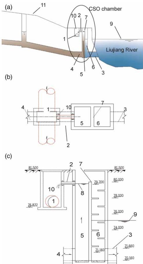
**Figure 1** | The deep CSO chamber in the intercepting sewer system in Liuzhou, China. (a) Panorama; (b) plan view; (c) cross-section view with the installation of SSCS. 1. main intercepting sewer; 2. branch intercepting sewer; 3. combined sewer outlet; 4. combined sewer channel; 5. overflow chamber; 6. discharge chamber; 7. weir; 8. intercepting water level; 9. water level of receiving water; 10. intercepting chamber; 11 ground.
