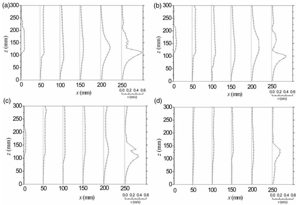
Figure 4 | The vertical distribution of time-averaged velocity in the xz-plane ( $y = 0$ ) with  $h = 0.75$  m (a),  $0.60$  m (b),  $0.45$  m (c) and  $0.30$  m (d).
