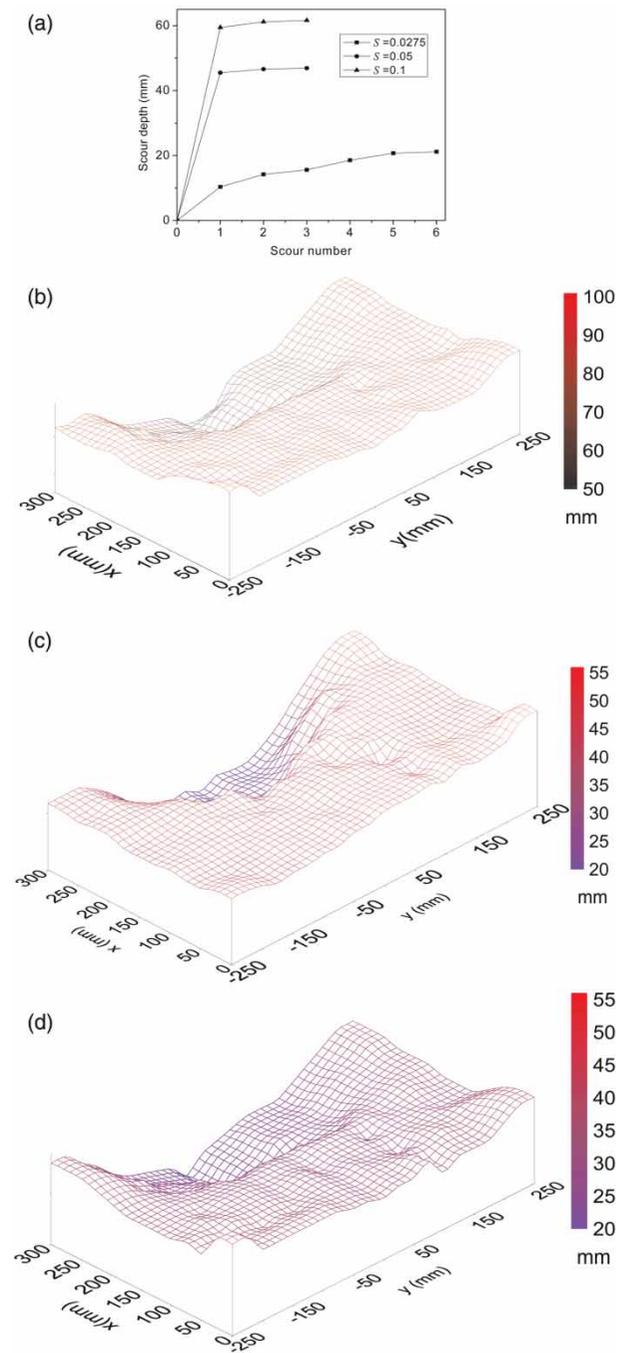
Figure 6 | The averaged scour depths on the bottom of the overflow chamber (a) and equilibrium sediment surface shape on the bottom as  $S = 0.0275$  (b), 0.05 (c) and 0.1 (d).
