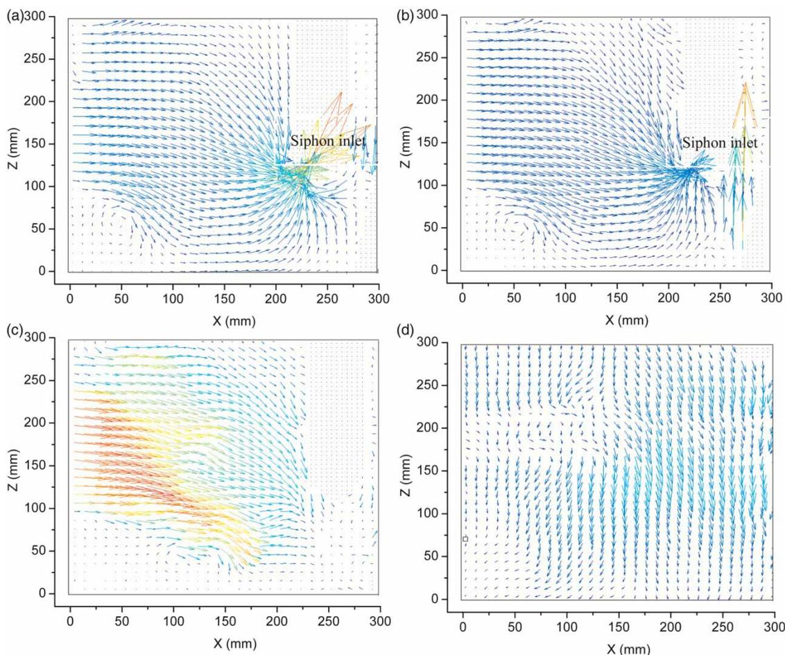
**Figure 3** | Time-averaged velocity fields on the bottom of the overflow chamber with siphon sediment cleansing set (a)  $y = 0$ , (b)  $y = 50$ , (c)  $y = 100$ , (d)  $y = 150$ .
