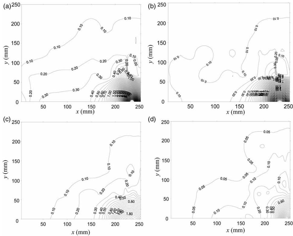
Figure 5 | The bed shear stress ( $xy$ -plane,  $z = 0$  mm) of the overflow chamber with SSCS under a different water head (a)  $0.75$  m, (b)  $0.60$  m, (c)  $0.45$  m, (d)  $0.30$  m.
