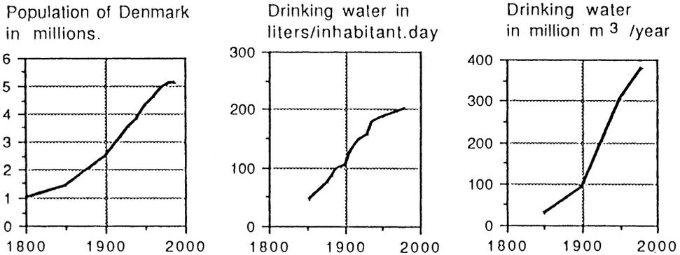
Fig. 2. The consumption of drinking water in Denmark.
