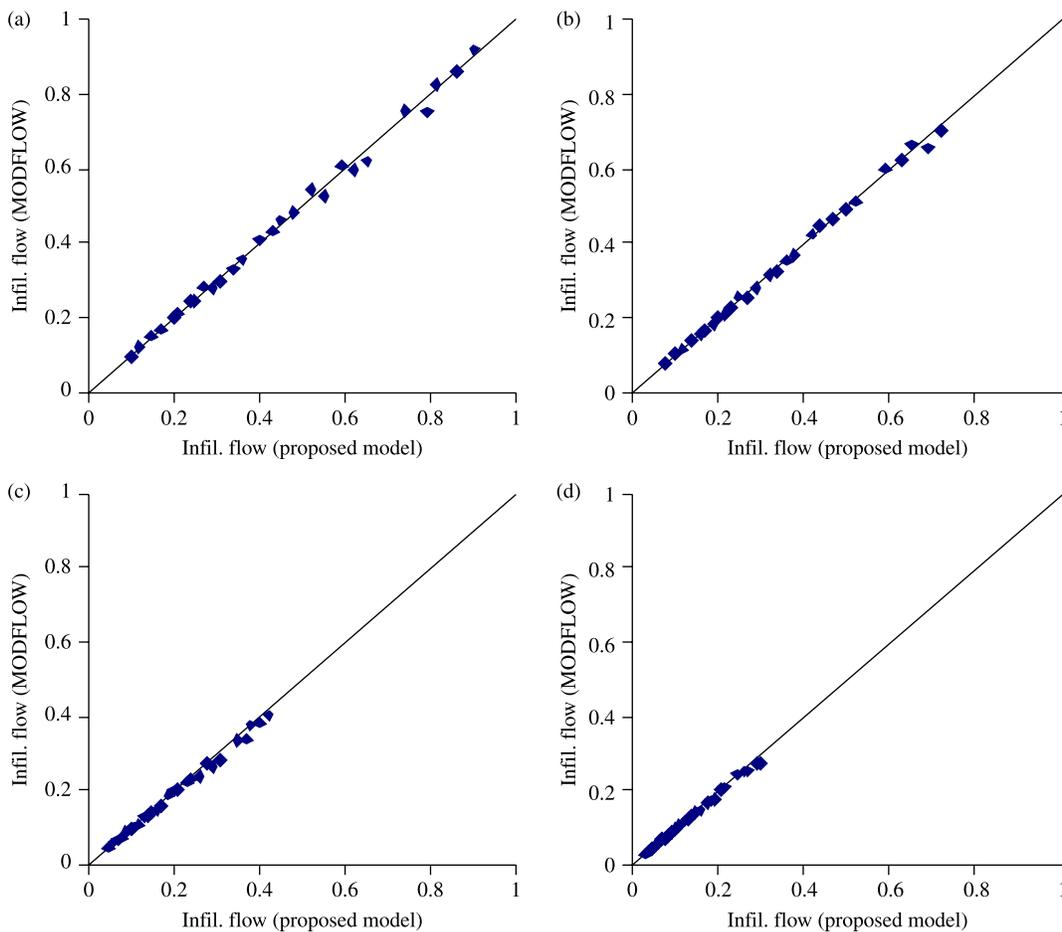
**Figure 5** | Calibration of the regression curves for the clean infiltration structure (a) and for three sediment levels:  $h_{\text{SED}} = 0.1$  m (b);  $h_{\text{SED}} = 0.3$  m (c);  $h_{\text{SED}} = 0.5$  m (d). Curves are referred to sandy-loam and infiltration flow expressed in L/s.
