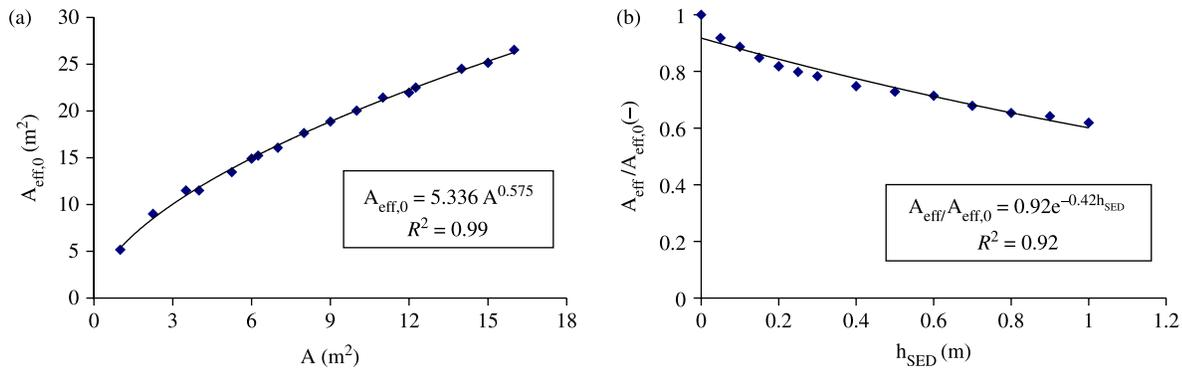
**Figure 4** | Correlation curves between (a) effective infiltration area  $A_{\text{eff},0}$  and geometric infiltration trench bottom area, in clean structure conditions and (b) effective infiltration area  $A_{\text{eff}}$  and sediment height, in clogging condition; curves are referred to sandy-loam.
