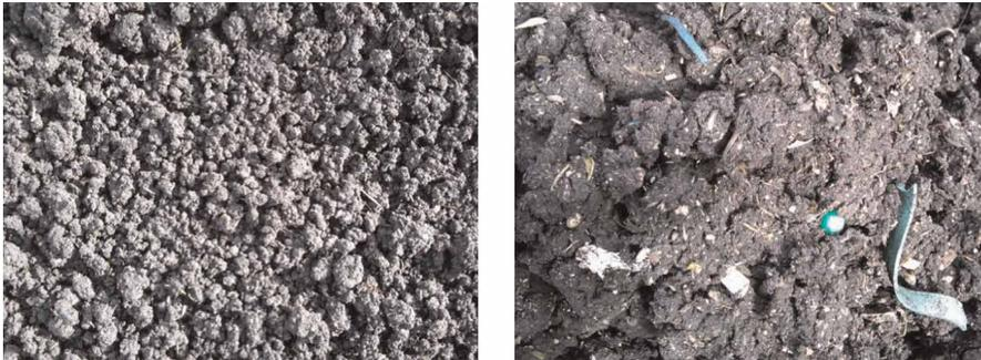
**Figure 3** | (Left) Pre experiment biosolids and (Right) biosolids centrifuged during the course of the experiment.
