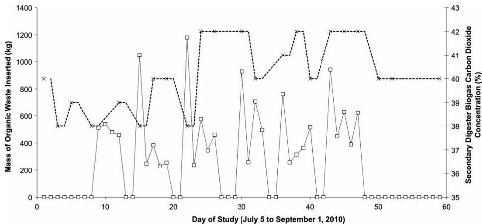
**Figure 2** | Primary and secondary digester biogas carbon dioxide concentration over the course of the study (July 12–August 20, 2010). Dashed line represents carbon dioxide concentration. Solid line indicates the mass of FFW inserted.
