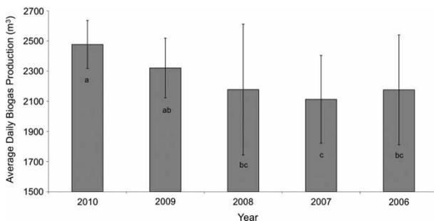
**Figure 1** | Average daily biogas production during the addition of FVW (July 12–August 20, 2010) compared to previous years without addition. (Means with the same letter are not significant at  $p < 0.05$ .)
