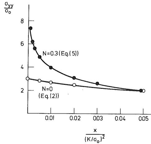
Fig. 1 Stress distribution ahead of crack
