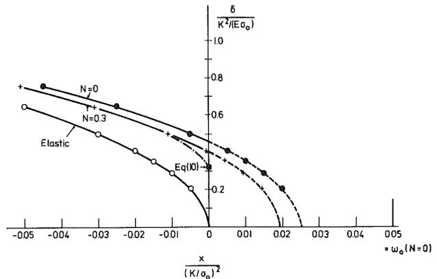
Fig. 2 Calculated crack tip profiles
