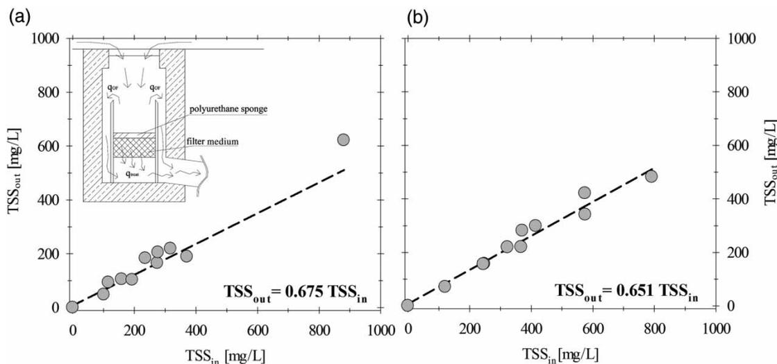
**Figure 2** | Influent and effluent PM concentrations (expressed as TSS) for catch basin (a) and catch basin (b). In the inset,  $q_{\text{or}}$  and  $q_{\text{treat}}$  represent the overflow flow rate and the treated flow rate, respectively.
