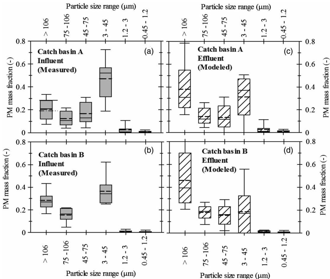
**Figure 1** | Measured influent (a), (b) and modeled effluent (c), (d) PM mass fraction for six particle size ranges for catch basin A and catch basin B. For each particle size range the median value (continuous black line) and the mean value (dashed line) are reported. In addition to the median and mean values, the box plots indicate the percentiles of 5, 25, 75, 95. The statistics are based on a sample size of 10 hydrological events.
