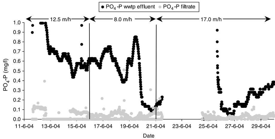
**Figure 3** Phosphorus removal during simultaneous denitrifying multi-media filtration (dosing of 1.5 mgAl<sup>3+</sup>/l)
