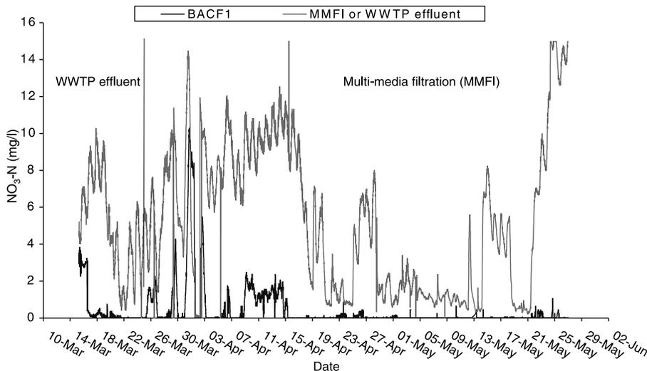
**Figure 4** NO<sub>3</sub>-N concentrations for biological activated carbon (van Oene, 2004)
