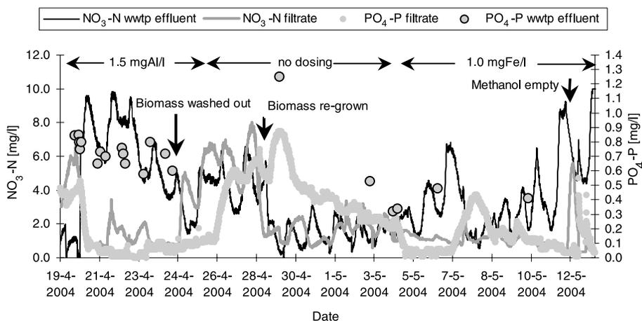
**Figure 2** Nitrogen and phosphorus removal during simultaneous denitrifying multi-media filtration
