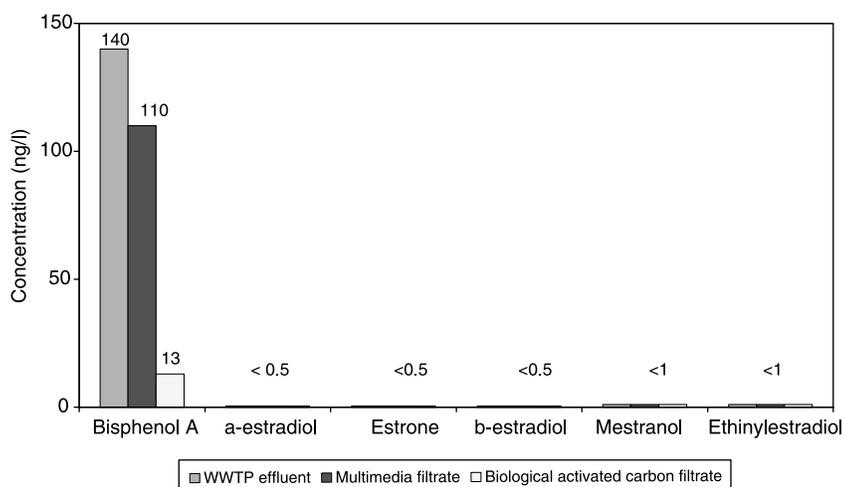
**Figure 5** Removal efficiency for biological activated carbon (Menkveld, 2004)
