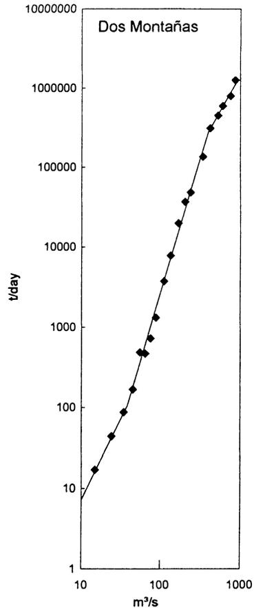
Fig. 3. Dos Montañas. Mean load in water discharge classes. Back-transformed log regressions corrected for bias by the correction factor  $10^{1.1513\sigma^2}$
