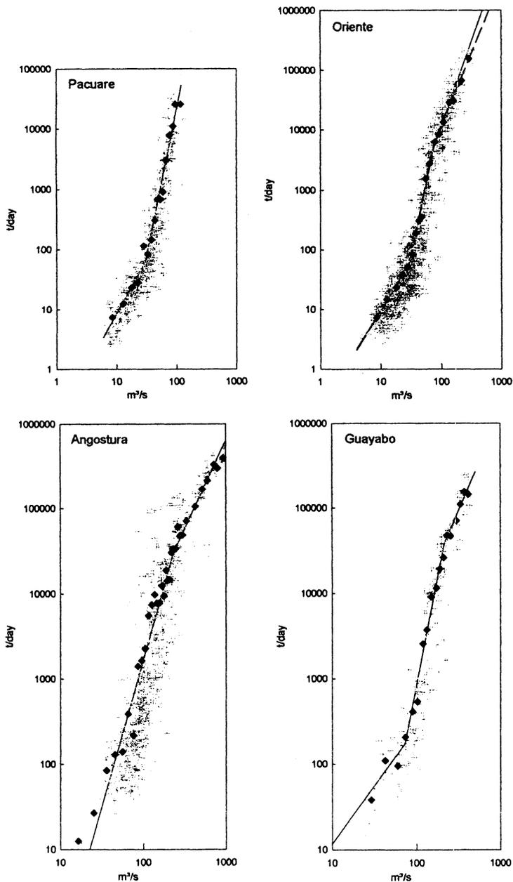
Fig. 4. Sediment rating curves developed on all separate values (crosses). Here these sediment rating curves are compared with the arithmetic mean values of load within water discharge classes. A second sediment rating curve developed on mean loads for individual discharge classes is marked on the diagram of Oriente (hatched line).
