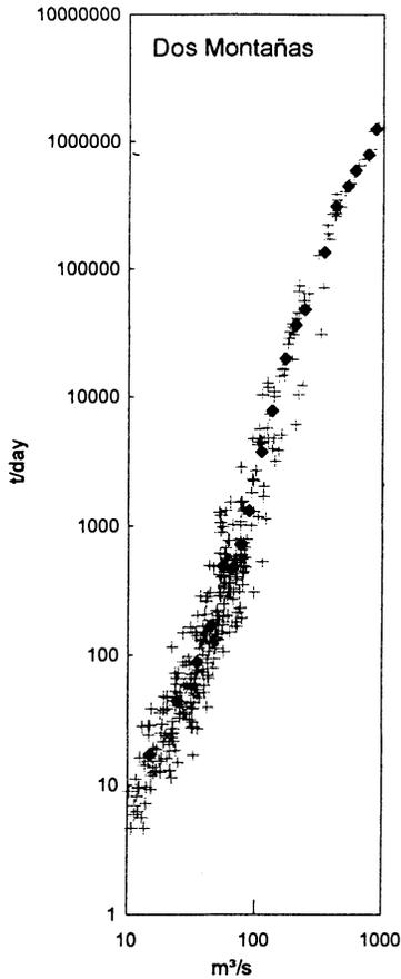
Fig. 2. Dos Montañas. Measurements made during 1970-1993. Samples are also taken during the passage of some highwater events in 1993-94. Mean loads for discharge classes.
