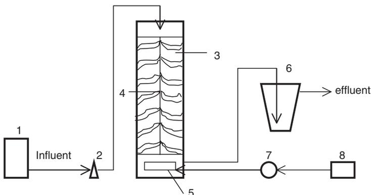
**Figure 1** Schematic diagram of a FFBR System (1: Equilibrium Tank, 2: Peristaltic Pump, 3: FFBR, 4: Fibre Packing, 5: Air Diffuser, 6: Settling Tank, 7: Air Flow Meter, 8: Air Compressor)
