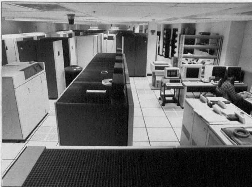
Cornell's IBM-FPS system offers scalar, vector, and parallel processing.
