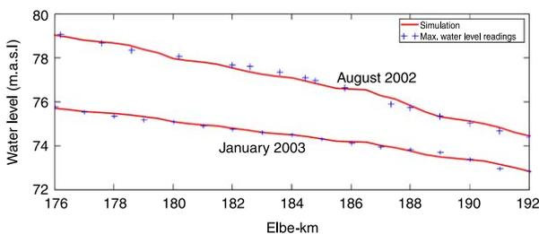
**Figure 5** | Longitudinal profiles of the simulated and recorded values of the highest water levels attained along Elbe 176–192 km during the August 2002 flood event (validation) and the January 2003 flood event (calibration).
