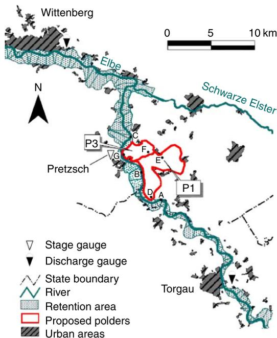
**Figure 2** | Researched river section and polders along the middle reach of the River Elbe in Germany between Torgau and Wittenberg (source: IWK 2004). Points A–G are the researched locations in the river and polders.
