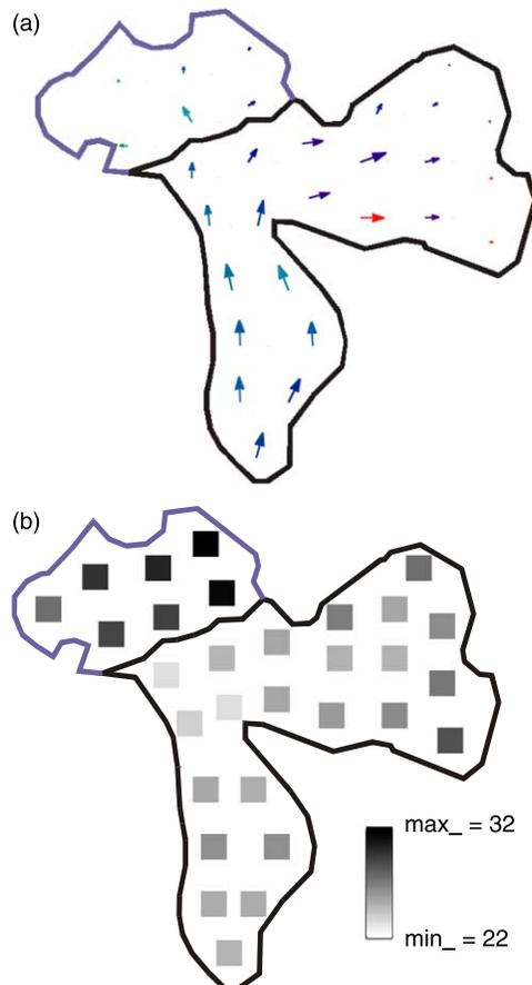
**Figure 11** | (a) Vectors of flow velocities during filling of the polder system on day 4.5; the longest vector corresponds to a magnitude ca. 1.2 m/s. (b) Reduction in particulate zinc concentrations ( $\mu\text{g/L}$ ) during flood water retention on day 8.5.
