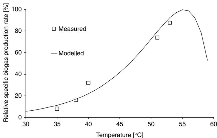
Figure 3 Modelled and measured relative specific biogas production rate
