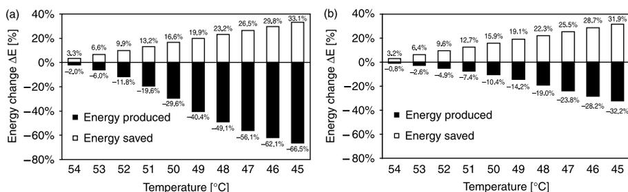
**Figure 4** Modelled change of energy at different temperatures for (a) faecal sludge treatment and (b) digestion of the model substrate
