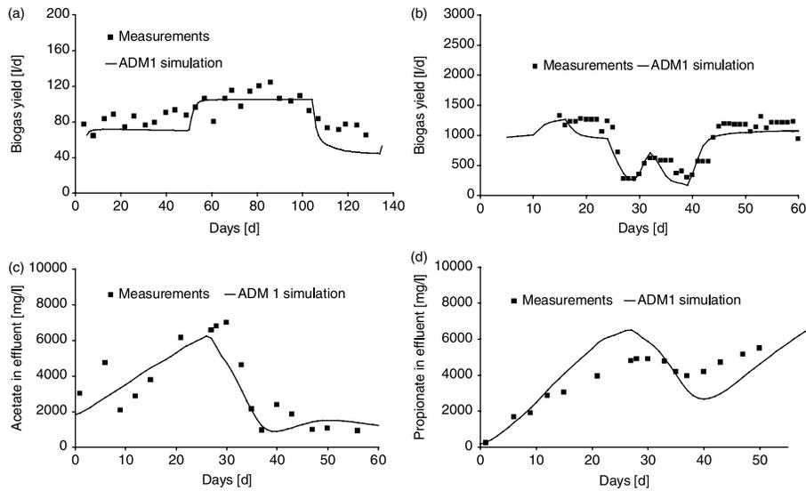
**Figure 2** Comparison of measurements and ADM1 simulation results for (a) faecal sludge treatment and (b–d) digestion of the model substrate
