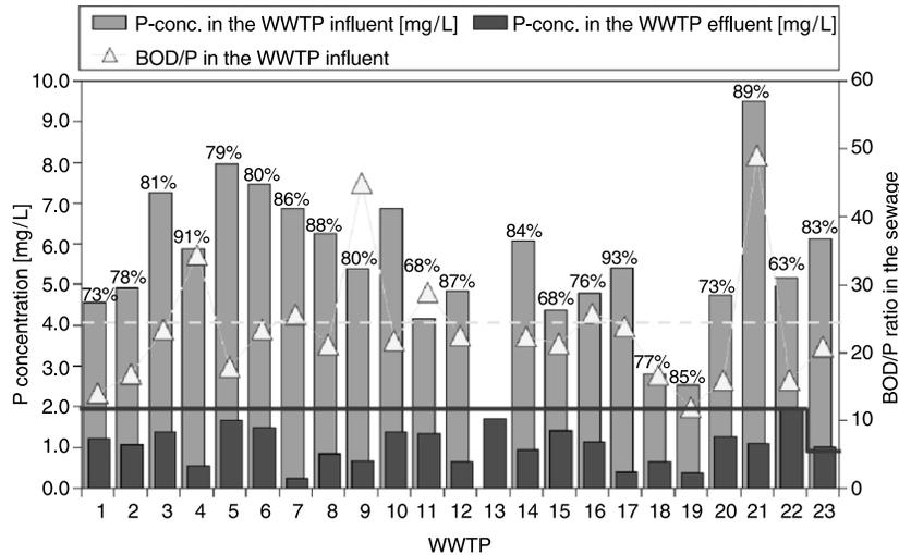
**Figure 1** Yearly-average phosphorus concentration in the influent and in the effluent and BOD<sub>5</sub>/P in the influent (secondary Y-axis) of the Flemish WWTPs using EBPR in 2003
