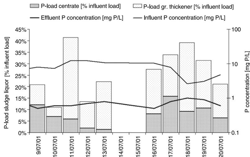
**Figure 2** Influent and effluent P concentrations and portion of the influent P load originated from the sludge liquors at the leper EBPR scheme in the period 9–20 July 2001.
