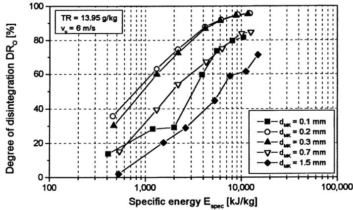
Figure 5 shows disruption results for constant solid content SS and circumferential velocity  $v_c$ . An optimum for the stress intensity can be detected for both specific energies. With the same specific energy a higher degree of disintegration can be achieved. Operating stirred ball mills with an optimum stress intensity reduces the energy cost.
