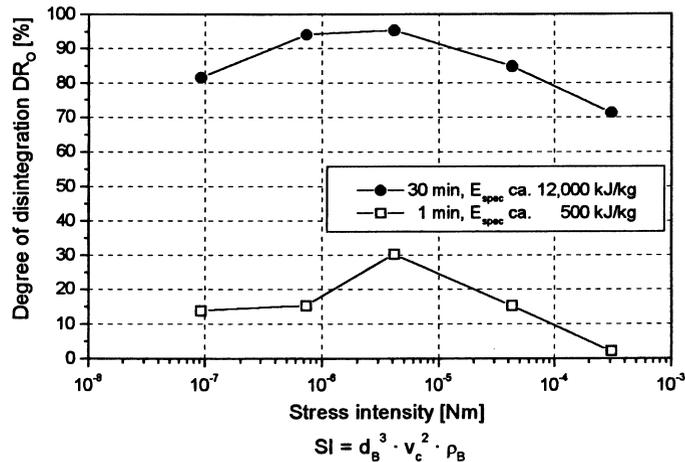
Figure 6 Influence of stress intensity on degree of disintegration for two specific energies
