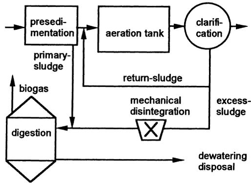
Figure 1 Flow sheet of a waste water treatment plant with mechanical disintegration of excess sludge
