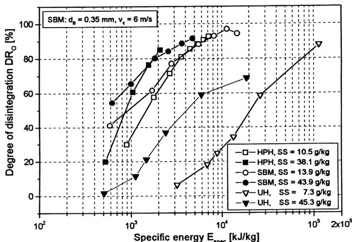
Figure 7 Comparison of different disintegration methods
