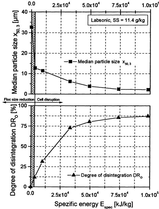
Figure 2 Degrees of disintegration and particle size for an ultrasonic disintegration
