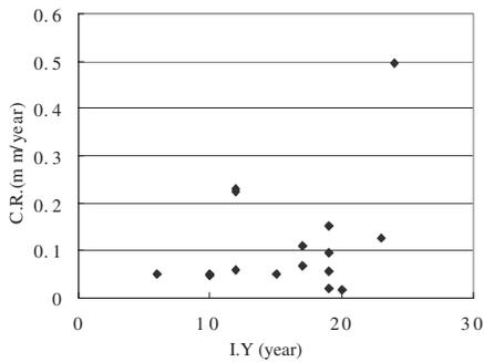
**Figure 8** Relationship between corrosion rate and installation year
