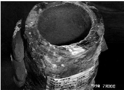
**Figure 1** Photograph of phenolphthalein test of DCIP
