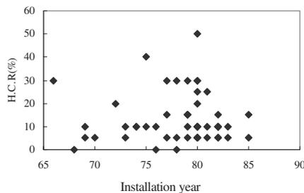
**Figure 4** Hydraulic capacity reduction analysis using CIP
