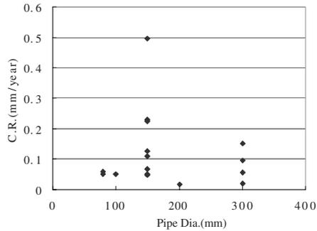
**Figure 9** Relationship between corrosion rate and pipe diameter
