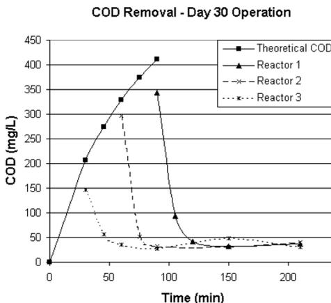
**Figure 1** Initial COD at the beginning of React and COD removal during one cycle
