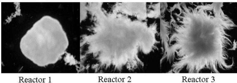
**Figure 4** Images of aerobic granules cultivated in each reactor (Reactor 1, 2 and 3 with 0%, 33% and 66% Aerated Fill, respectively). Taken approximately 60 days after start-up
