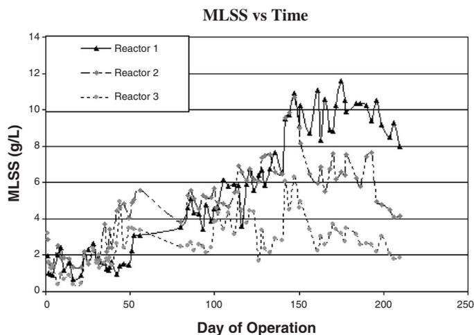
**Figure 2** MLSS for Reactors 1, 2, and 3 over time
