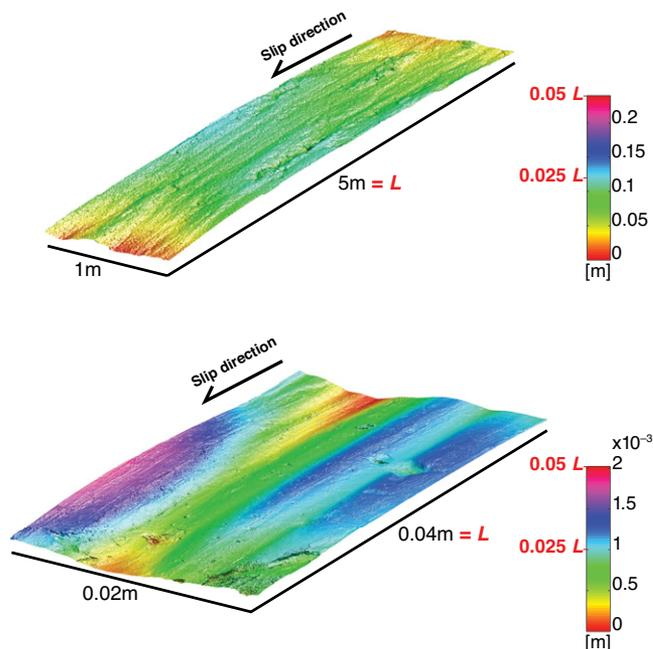
**Figure 2.** Fault patches of the Corona Heights fault (California, USA) demonstrating the scale-dependent roughness behavior in the spatial domain. For each fault patch (lidar at the top and laser profilometer at the bottom), the maximum of the color scale (red) is set to be equal  $0.05 L$ , the measured patch length in the slip direction. At the lidar scale (top), the roughness magnitude reaches only  $\sim 0.01 L$ , whereas at the laser profilometer scale, it reaches  $\sim 0.05 L$ .
