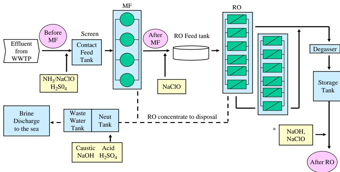
**Figure 1** | Schematic representation of the advanced treatment at KWRP and BPP. Sample points represented by circles. Note: \* There is no post-RO chemical dosing at the BPP.
