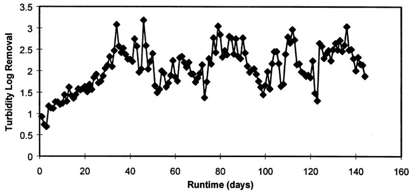
Fig. 6 Plot of turbidity log removal vs. cumulative run-time with associated turbidity data collection.
