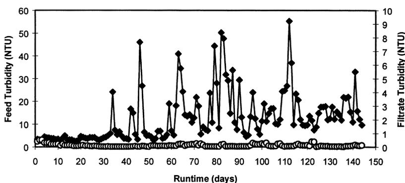
Fig. 5 Plot of average feed and filtrate turbidity vs. cumulative run-time with associated turbidity data collection.
