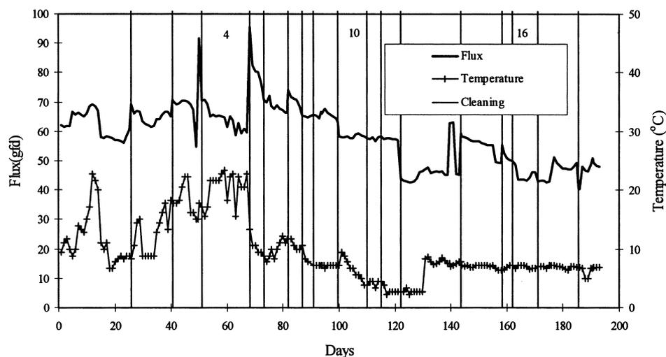
Fig. 2 Temperature, flux, and cleaning interval vs. operating time.
