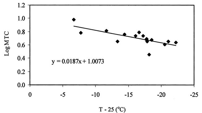
**Fig. 1** MTC vs. temperature for operational data.
