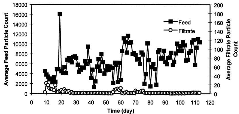
**Fig. 7** Plot of particle count for raw feed and filtrate vs. consecutive day of particle count data collection.
