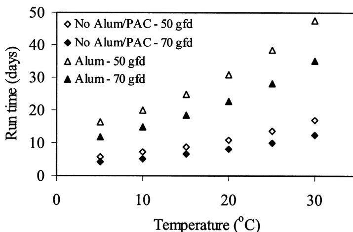
Fig. 4 Run time vs. Temperature for varying flux for No alum-PAC, and for Alum.
