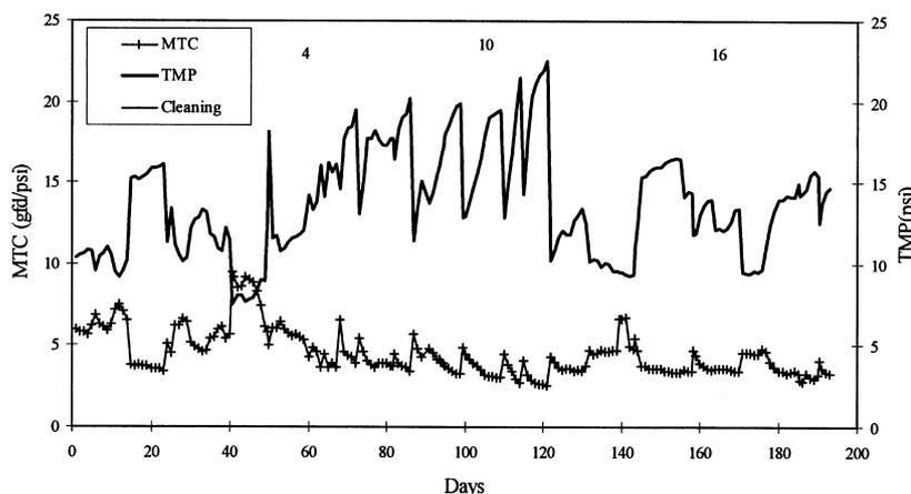
Fig. 3 Transmembrane pressure, mass transfer coefficient and cleaning interval vs. operating time.
