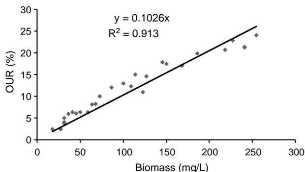
Figure 3 Relationship between oxygen consumption and biomass
