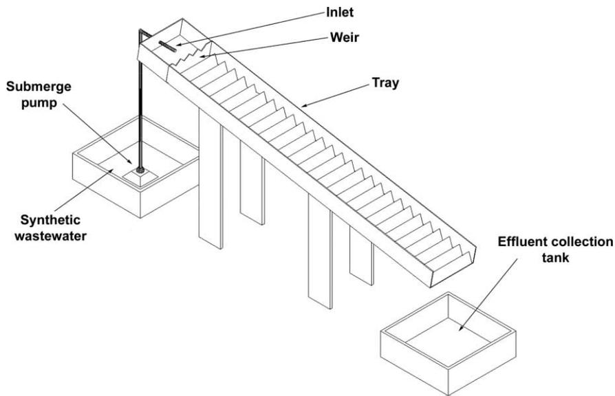
**Figure 1** Experimental setup of lab-scale ACSB
