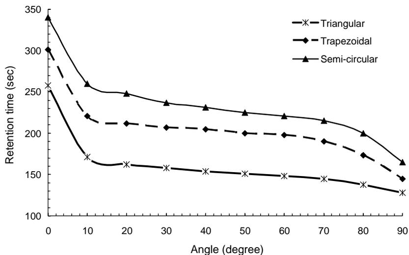
**Figure 6** Comparison of hydraulic retention time at different sponge shape and inclination slope of sponge tray
