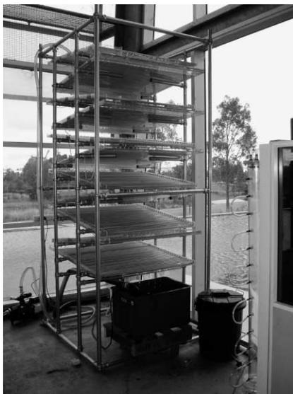
**Figure 2** Experimental setup of pilot-scale ACSB at a water reclamation plant
