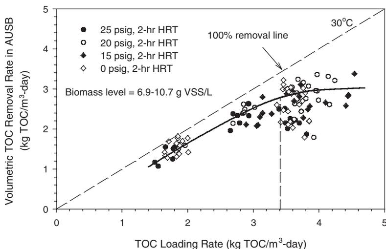
**Figure 3** Effect of loading on substrate removal rate
