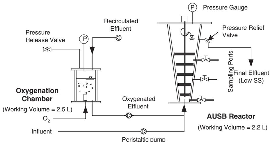
**Figure 1** Schematic of the AUSB reactor set-up
