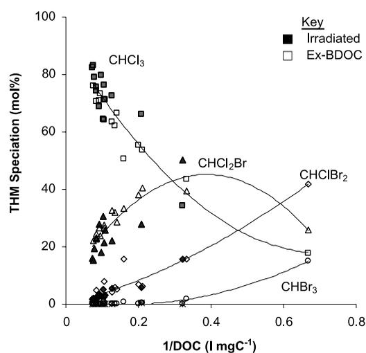
**Figure 6** | THM speciation of Myponga water after various treatments. Symbols show experimental data. Trendlines also shown. There was little variation in THM speciation between the irradiation treatments and in the interests of clarity N-lamp, H-lamp, N-lamp/ $\text{H}_2\text{O}_2$  and H-lamp/ $\text{H}_2\text{O}_2$  data points are not distinguished and are shown as filled symbols.
