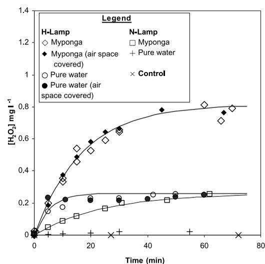
**Figure 3** | Formation of  $\text{H}_2\text{O}_2$  by irradiation. The control was Myponga water aerated in the reactor without irradiation. Symbols show data and lines are trendlines.
