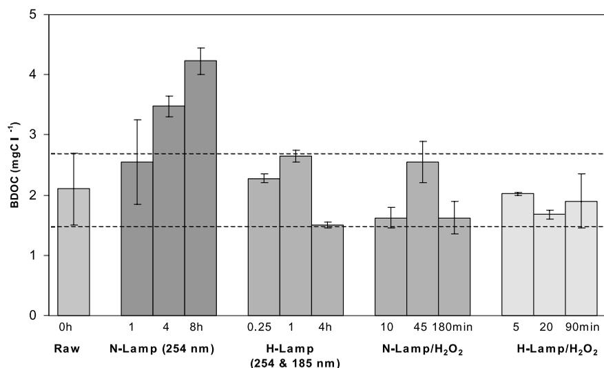
**Figure 4** | Effect of irradiation on biodegradability. Averages of duplicates shown here with difference between duplicates indicated by uncertainty bars.
