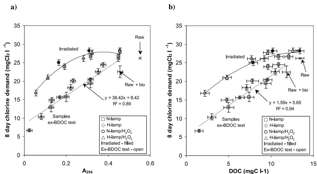
**Figure 5** | Effect of treatment on chlorine demand. Degree of treatment indicated by (a) absorbance ( $A_{254}$ ) and (b) DOC. Average of duplicates shown.
