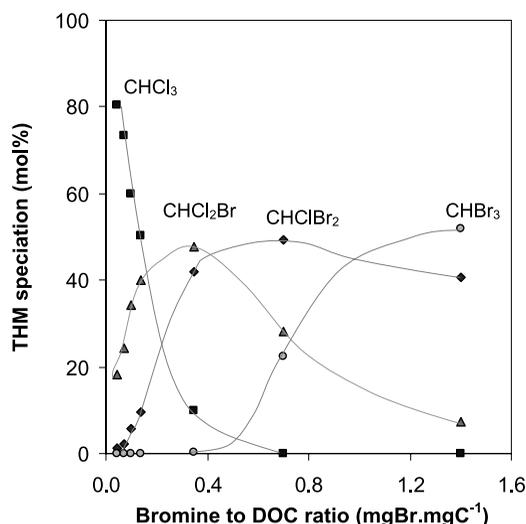
**Figure 7** | Effect of bromine:DOC ratio on THM speciation in chlorinated Aldrich humic acid solutions. Bromide concentration constant at  $0.7 \text{ mg l}^{-1}$ , DOC varied from  $0.5$  to  $15 \text{ mgC l}^{-1}$ . Hypochlorite added in excess at  $5 \text{ mgCl}_2 \cdot \text{mgC}^{-1}$ .
