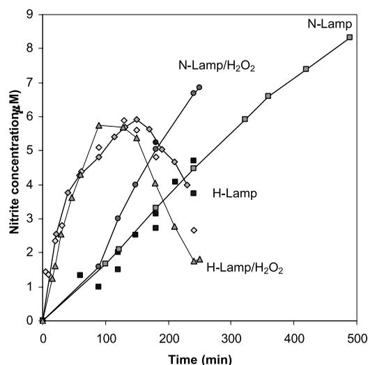
**Figure 9** | Nitrite formation in irradiated Myponga water. Symbols show experimental data points; lines added to guide the eye.
