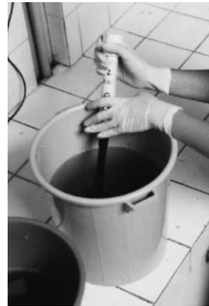
**Figure 4** | Washing of the sand layers.
