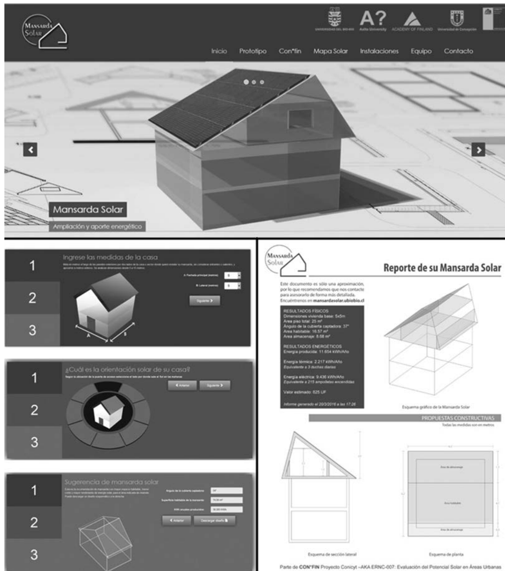
FIGURE 7. Solar attic website, main screen (upper), design steps (lower left) and report generated (lower right).
