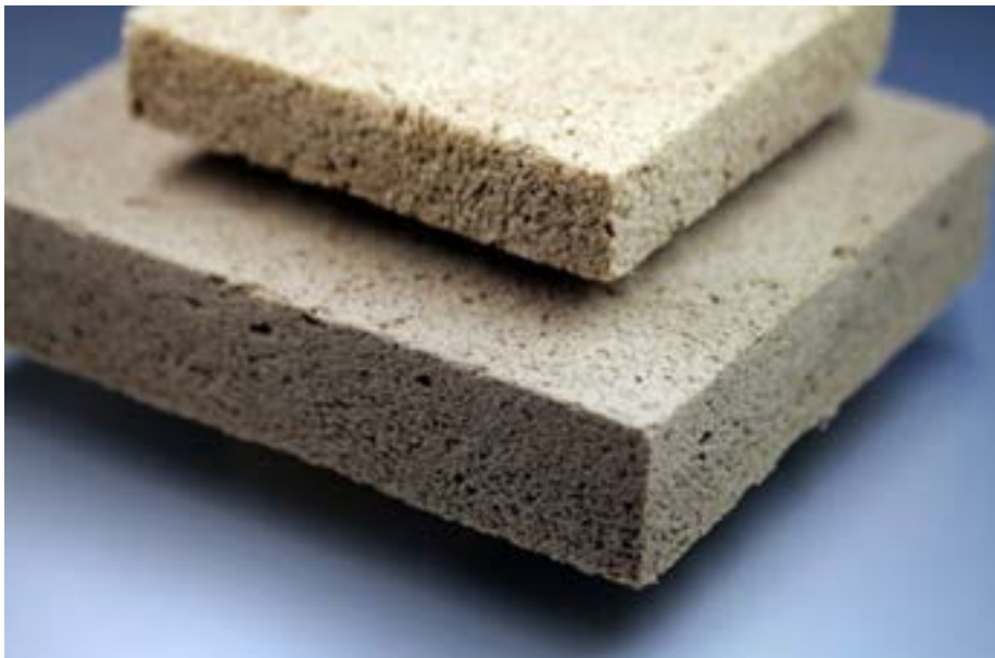
FIGURE 6. The wood spray solidifies, forming totally biodegradable insulating panels
