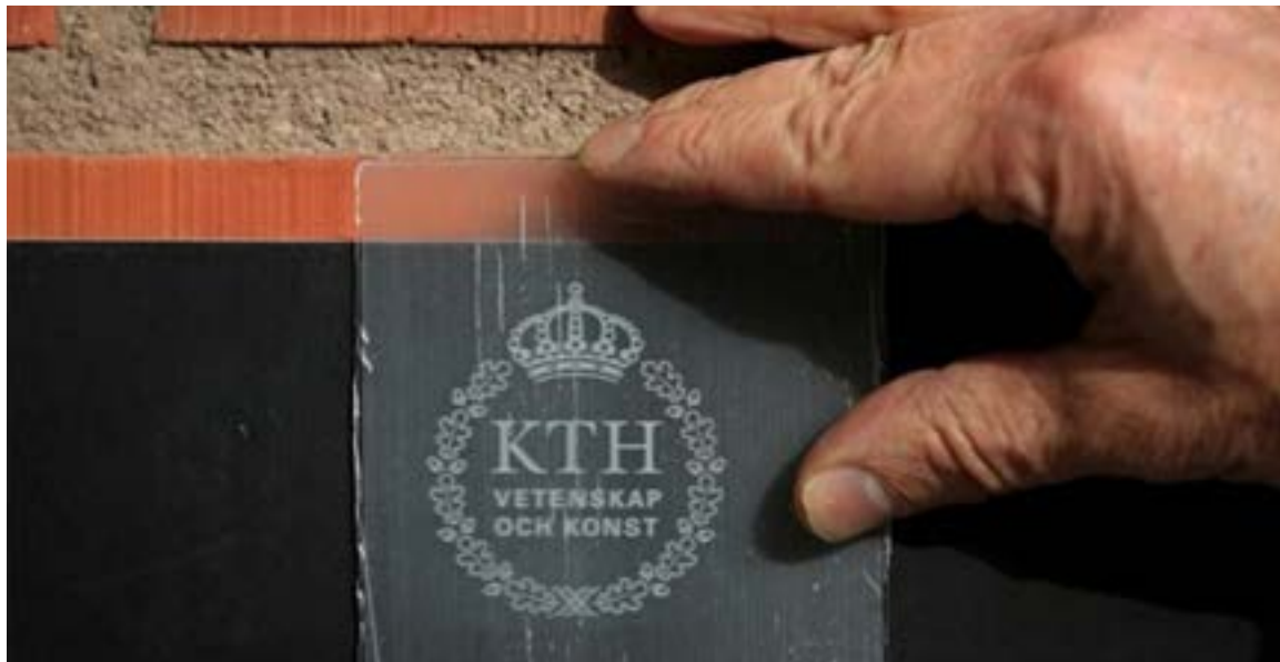
FIGURE 8. A close-up look at the transparent wood created by Dr. Lars Berglund and co-authors
