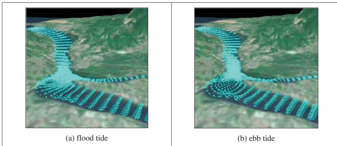
**Figure 4** | Model-predicted flow currents at flood and ebb, respectively.
