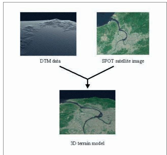
Figure 2 | Construction of the terrain model of Tamshui River Basin.
