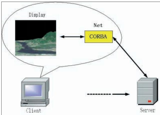
**Figure 7** | Architecture of collaborative visualization environment.
