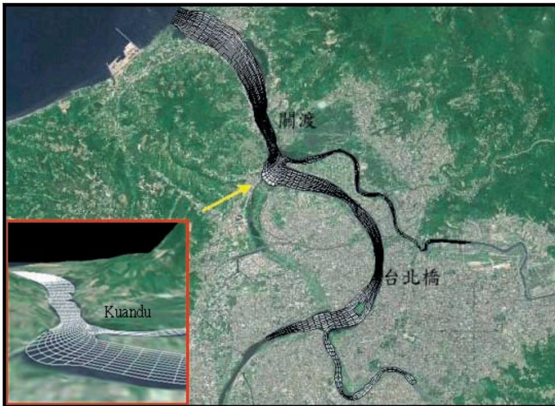
Figure 3 | Grid configuration for Tamshui River.
