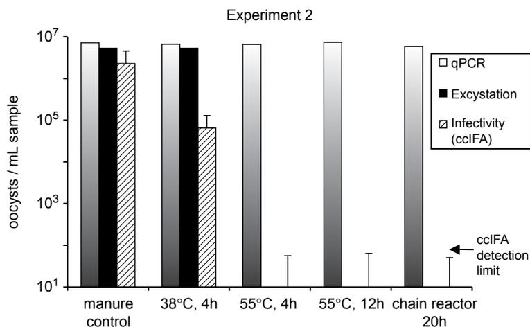
**Figure 2** Effect of different anaerobic digestion conditions on *C. parvum* oocysts as determined by qPCR, excystation rate and infectivity test (cell culture immunofluorescence assay) after percoll gradient purification; h: hours
