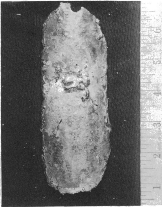
Fig. 2 Window sample from furnace A is approximately 2 in. x 6 in. The longer length is the longitudinal direction (parallel to tube axis). The creep rupture test specimens were prepared so that the circumferential direction was tested.
