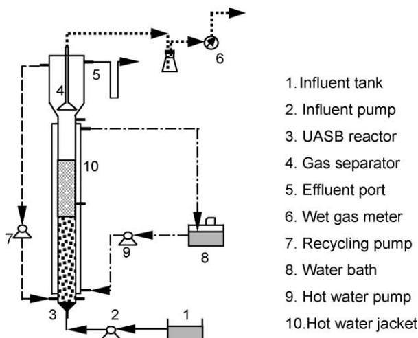
**Figure 1** Experimental apparatus and process scheme chart
