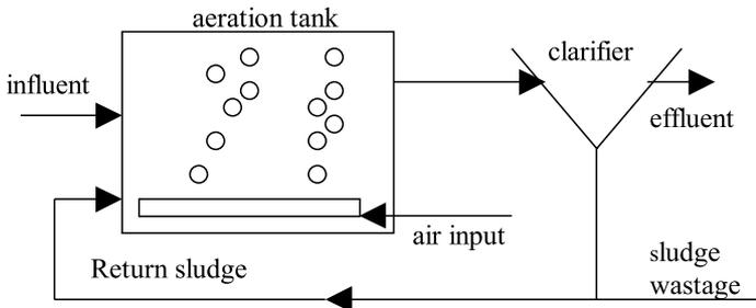
Figure 1 Sewage treatment plant flow sheet
