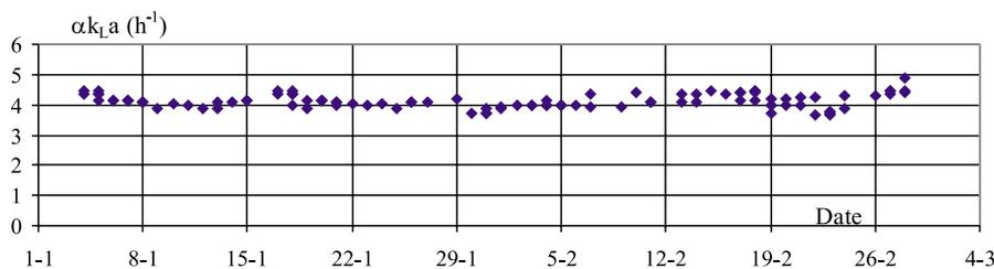
Figure 4 Evolution during the test week (one blower instead of two) of estimated  $\alpha k_L a$
