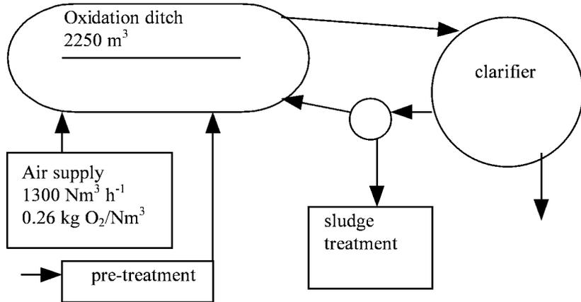
Figure 2 Wastewater treatment plant A flow sheet
