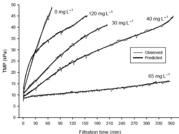
**Figure 5** | Sixth-degree bivariate polynomial fit of membrane fouling.
