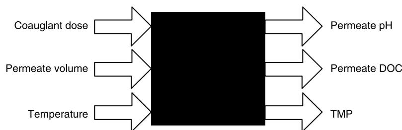
**Figure 1** | Conceptual model of the hybrid membrane system.
