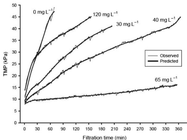
Figure 10 | GRNN model fit of membrane fouling using a spread value of 1.
