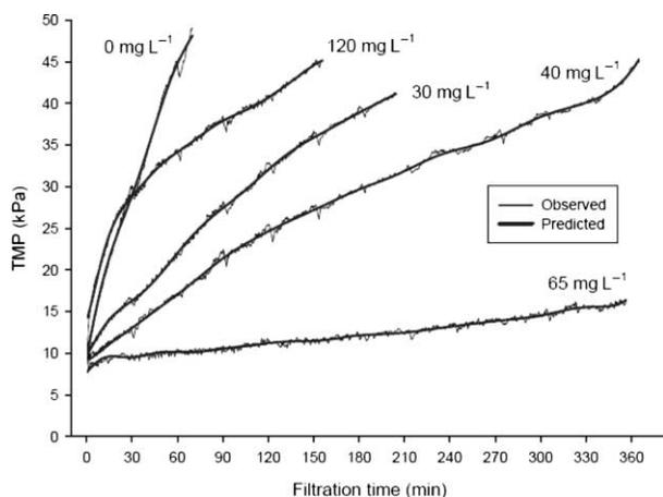
Figure 9 | RBF model fit of membrane fouling using 50 nodes and a spread value of 40.
