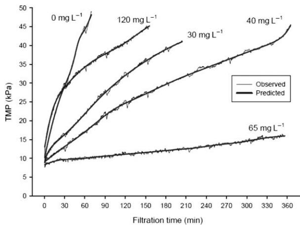
**Figure 8** | MLP model fit of membrane fouling using 15 nodes in the first, and 6 nodes in the second hidden layer.
