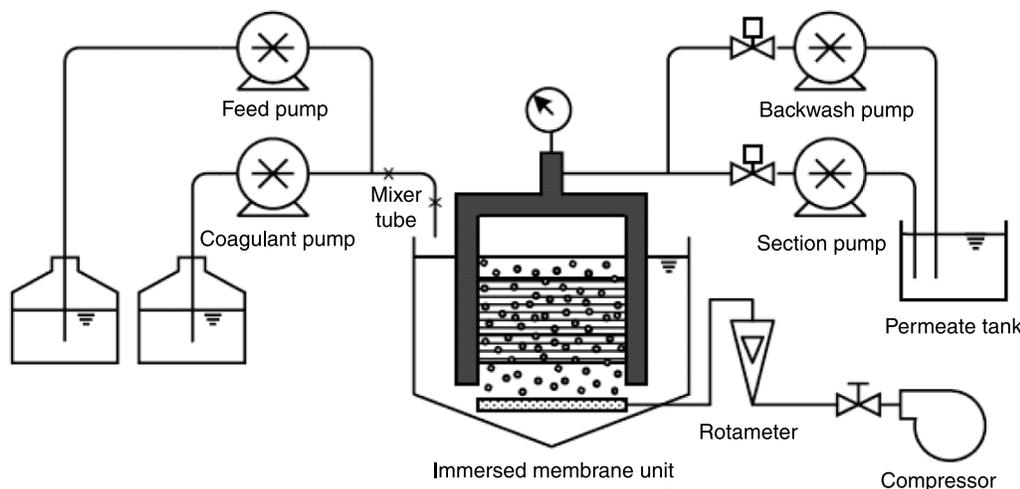
**Figure 3** | Schematic diagram of the experimental bench-scale hybrid in-line flocculation–membrane system.
