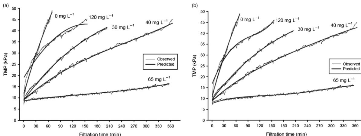
Figure 6 | Comparison of (a) second-degree bivariate polynomial fit, (b) sixth-degree bivariate polynomial fit of membrane fouling using stepwise regression.
