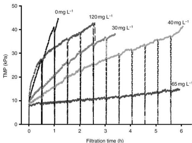
**Figure 4** | Membrane fouling at a constant flux of  $36 \text{ L m}^{-2} \text{ h}^{-1}$  (Mitsubishi  $0.1 \mu\text{m}$  pore size membrane) as a function of  $\text{FeCl}_3$  coagulant dosage used for in-line flocculation.**Table 3** | Permeate water quality data for the system model
