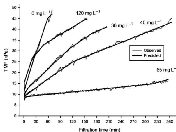
Figure 11 | Adaptive logic network model fit of membrane fouling with constrained training and single tree.
