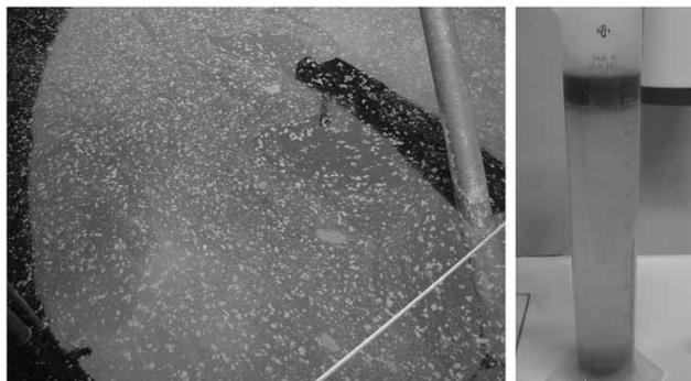
Figure 10 | Floating sludge in plant S during the conversion (left) and in the laboratory after 25 min of sedimentation (right).
