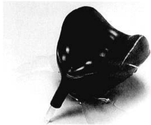
FIG. 1. The defective anesthesia mask with the rim cushion filled with fluid under pressure.
