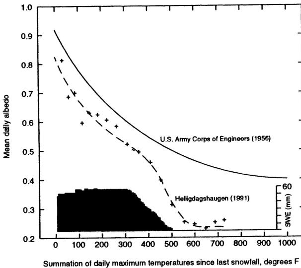
Fig. 5. Variation of albedo as a function of the accumulated daily maximum temperature index,  $T_{acc}$ . Temperature and albedo measurements for Helligdagshaugen are from April 16 through May 3. Snow water equivalents are shown as shaded area.
