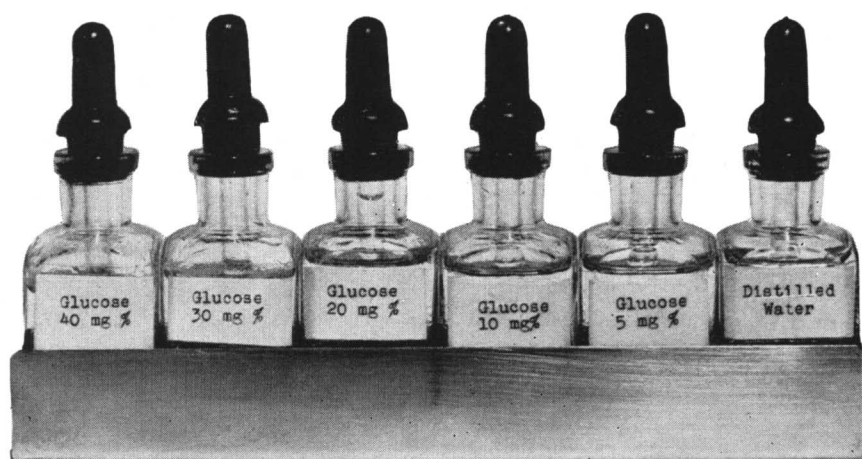
FIGURE 1. Rack with set of six drop- per bottles, five with glu- cose standard solutions and one with water.
