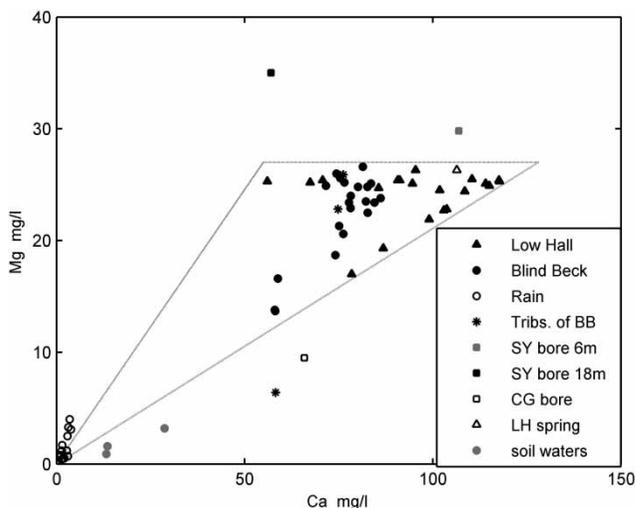
**Figure 4** | Concentration inter-relationship for magnesium (Mg) and calcium (Ca) for waters within the Blind Beck basin. The vertices of the dashed triangle indicate the calcium and magnesium concentrations of end-members.
