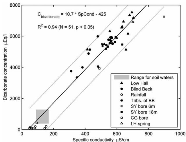
**Figure 6** | Concentration of bicarbonate (from charge balance) against specific conductivity, showing a linear relationship with coefficient of determination  $R^2 = 0.94$ . Number of samples,  $N = 51$ ; the relationship is significant at the 95% level ( $p < 0.05$ ). The grey lines show 95% confidence intervals on the regression.
