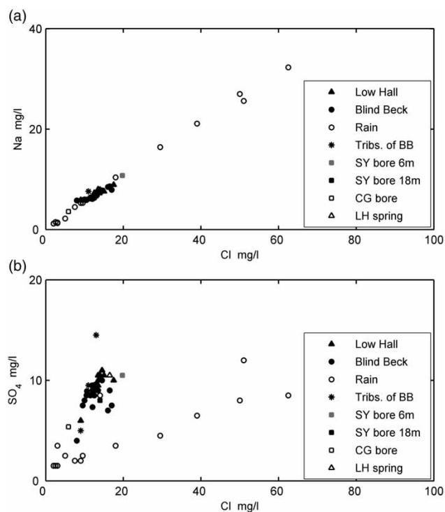
**Figure 3** | Concentration inter-relationships for (a) chloride (Cl) and sodium (Na), and (b) chloride (Cl) and sulphate (SO<sub>4</sub>) within the Blind Beck (BB) basin.
