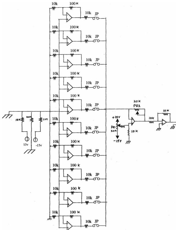
FIG. 4. Circuit diagram of a past preamplifier.
