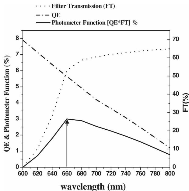
FIG. 3. The response function of the photometer.
