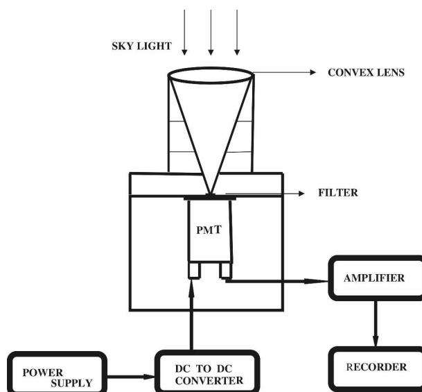
FIG. 2. Block diagram of the twilight photometer.
