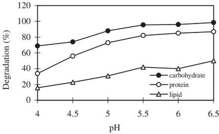
**Figure 1** Degradation of carbohydrate, protein, and lipid
