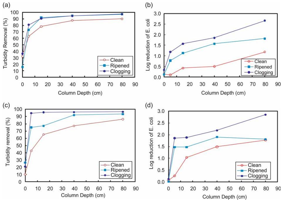
**Figure 5** | Example of turbidity and *E. coli* removal-with-depth profiles for sand and pumice media under different filter bed conditions of clogging; (a) and (b) pumice bed; (c) and (d) sand bed.
