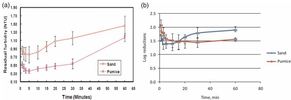
**Figure 7** | Temporal variation of filtrate quality during a typical charge: (a) turbidity; (b) *E. coli*.
