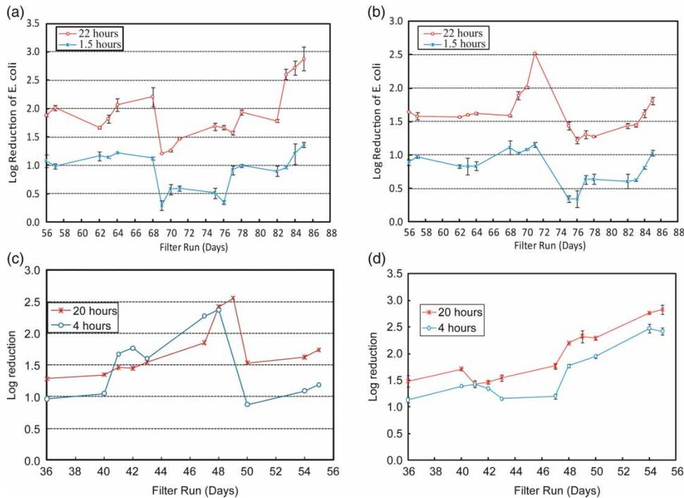
**Figure 6** | Influence of resting time on *E. coli* removal: (a) sand 1.5 and 22 h; (b) pumice 1.5 and 22 h; (c) sand 4 and 20 h; (d) pumice 4 and 20 h.
