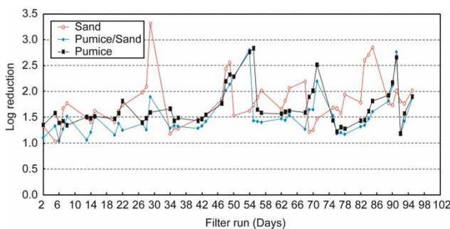
**Figure 4** | Variation of *E. coli* removal (logarithmic reduction) with filter run time over several filter cycles.
