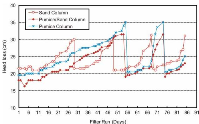
Figure 2 | Temporal variation of head loss curves for four consecutive filter cycles.
