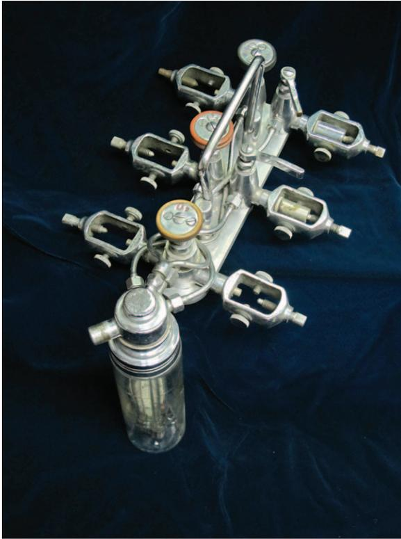
**Fig. 4.** Australian Foregger Midget machine. This machine is an earlier model with the water depression flowmeters enclosed in one tank (see fig. 5 for details of flowmeters). There are six yokes: two for oxygen, two for cyclopropane, and two for nitrous oxide and/or ethylene. Image courtesy of the Wood Library-Museum of Anesthesiology, Park Ridge, Illinois.
