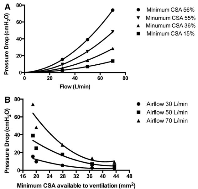
**Fig. 5.** (A) Pressure drop-flow curves in the tracheal tube *in vitro* experiments. Resistive curves of increasingly obstructed tracheal tubes were performed under condition of constant airflow. Minimum cross sectional area (CSA) is the percentage of CSA reduction compared with a never used tracheal tube of the same size; (B) nonlinear relationship between minimum CSA and the pressure drop to increasing airflow rates.
