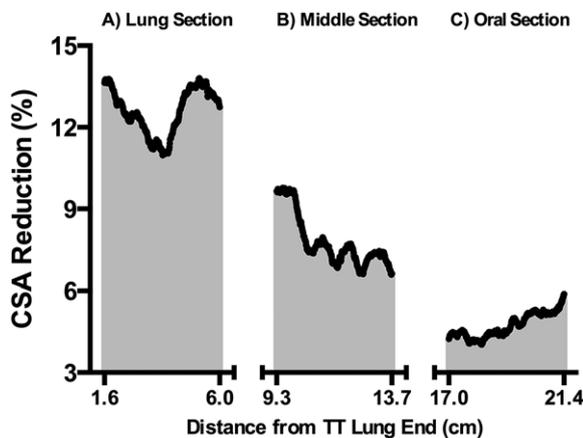
**Fig. 3.** Distribution of cross sectional area (CSA) reduction of used tracheal tube (TT) group along the tube length. Average CSA reduction for each slice of all used TTs is reported for each high-resolution computed tomography scan slice of the three TT sections: (A) lung end, (B) middle section, and (C) oral end of the TT. SD is not shown in the graph for clarity.
