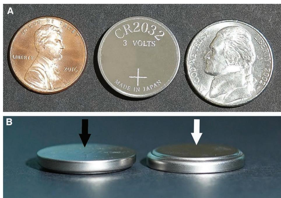
**Fig. 1.** CR2032 (20-mm diameter) lithium button batteries. (A) Size relationship to common U.S. coins. (B) Flat surface of positive battery pole (black arrow) on the left. Negative battery pole (white arrow) shown on the right with step-up to narrower flat surface.
