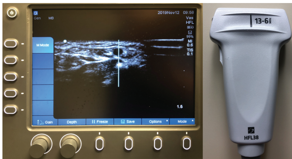
Fig. 1. In the left panel, the M-line is activated and centered through the radial artery. In the right panel, an HFL38x/13-6 MHz probe (FUJIFILM SonoSite, Inc., USA) is shown with its center marker, which can be used for final alignment.
