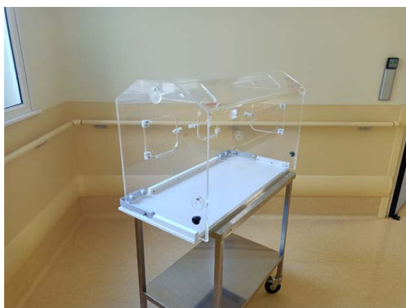
Fig 1. Neonatal plexiglass incubator hood (after removing one side and strengthening the base).
